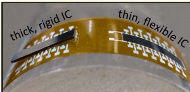
Comparison of conventional "thick" IC with a flexible thin one. The thick IC does not conform to the circuit board contour, nor is it connected at the edges.
